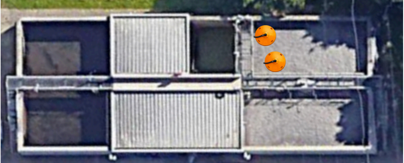
Figure 1: Aerial view of the investigated SBR with schematic hood placement
