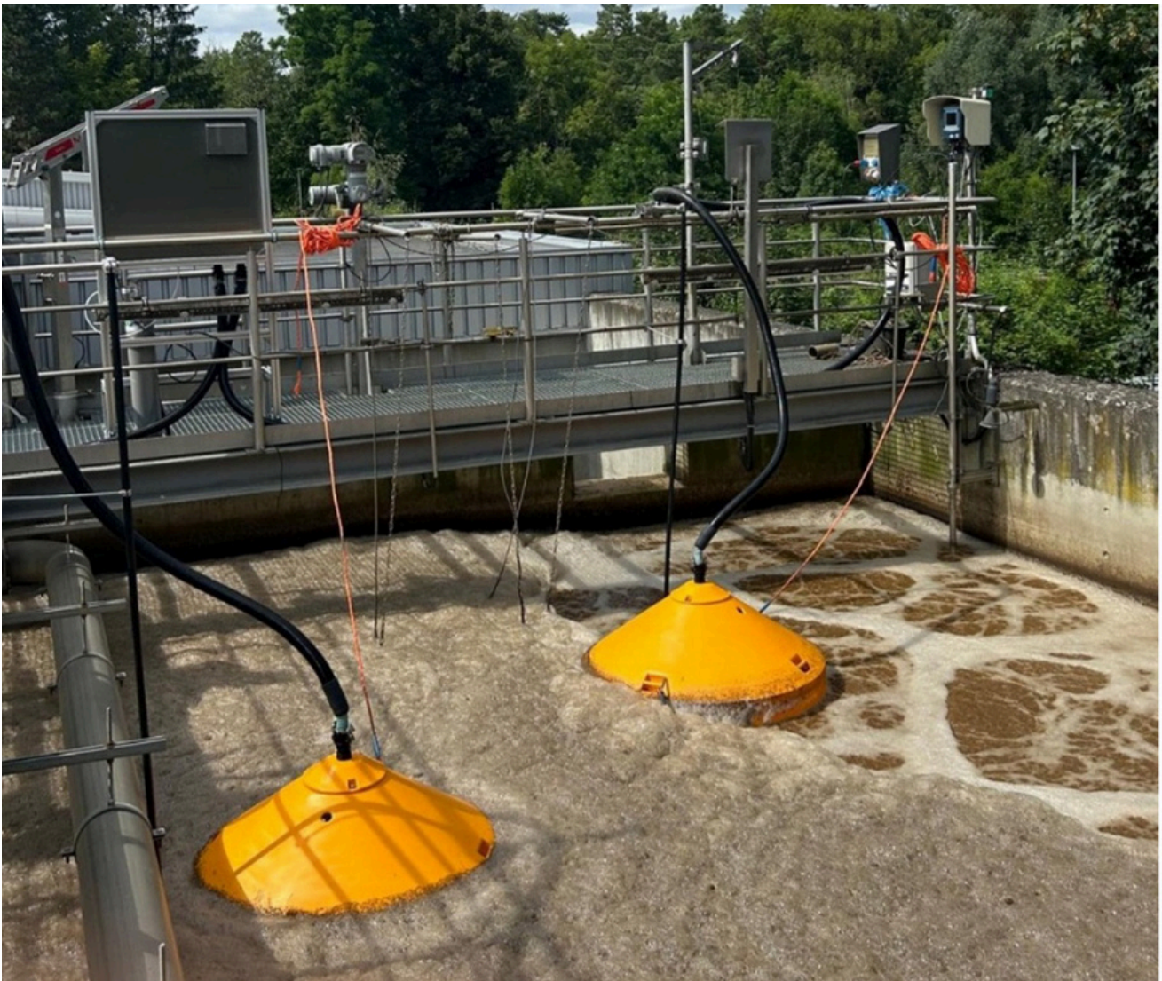
Figure 2: Setup of the EmiCo lite system at the investigated SBR.
